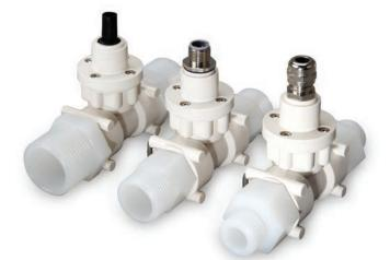
This multi-range radial flow turbine meter uses a low inertia turbine supported on robust sapphire bearings in a chemically resistant housing. 9 flow ranges (0.02 to 160 L/min), a choice of "plug in" fittings and individual traceable calibration make this meter one of the most flexible available. For OEM applications the fittings can be tailored to suit the installation and speed production. Custom leads or connectors are also available for quantity orders.
