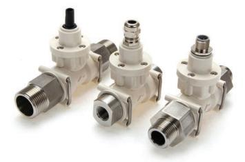
This multi-range radial flow turbine meter uses a low inertia turbine supported on robust sapphire bearings in a chemically resistant housing. Nine flow ranges (0.05 to 160 L/min), a choice of "plug in" fittings and individual traceable calibration make this meter one of the most flexible available.
