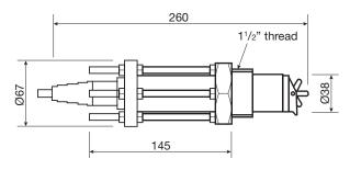
Insertion depth = pipe internal diameter divided by 8.
