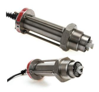
This innovative, robust insertion turbine combines proven technology with modern materials and design. The PVDF turbine rotates freely on a 316 St St shaft and has specially aerofoil shaped blades to extend the dynamic range of the meter. The specially contoured housing further improves the meters linearity particularly at lower fluid velocities. Each meter contains two sensors, one self powered for our battery operated equipment and the other an open collector transistor.
